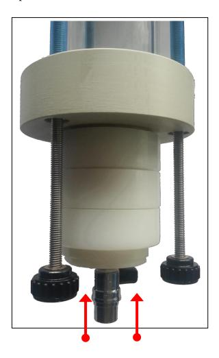
• Use the stainless steel plate shown in the figure below to lock down the membrane holders.
